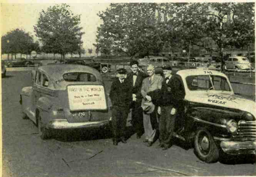
Two-way Motorola FM radio employing a wavelength of 118.65 mc. is now in use by Cleveland's Yellow Cab Company, to direct and control operations of fleet. One hundred additional cabs will be equipped pending permission by the FCC. Remote control station in dispatcher's office transmits messages to cabbies on the go. Power of 15 watts is used for both mobile and fixed transmitters.
